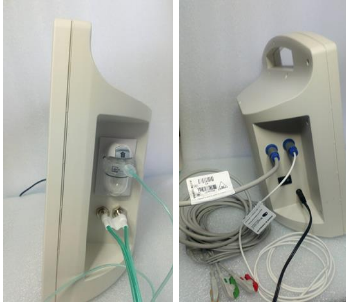
Figure 2. Sides of the device for the sensor and main power connection
