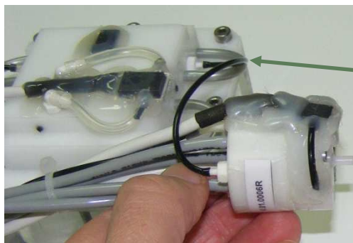
Pneumatic connection between the main pneumatic valve and the gas box
