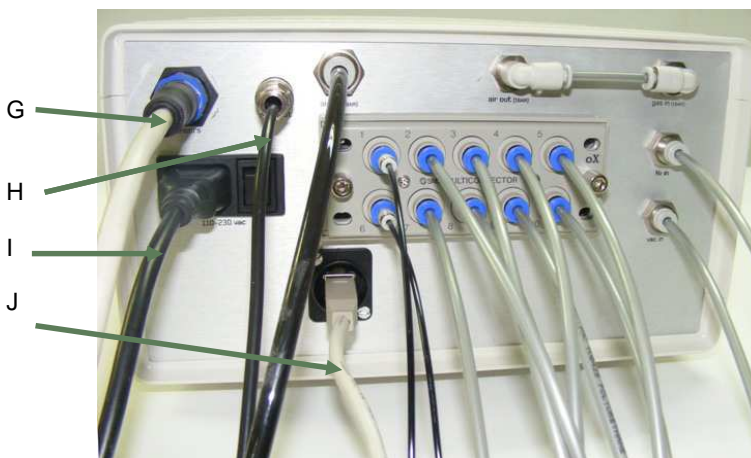
Picture of the back panel of device with the electrical and pneumatic connections
